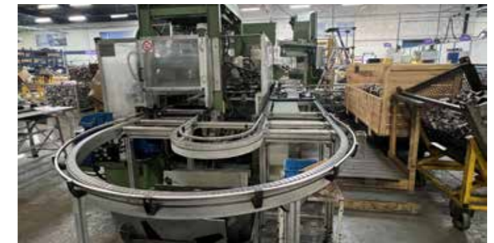
Spacer dampers automatic assembly line
